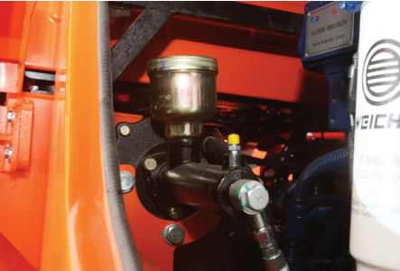
The booster pump delivers a higher augmented-thrust ratio, more stable braking performance, and more convenient daily maintenance thanks to its being mounted on the body's side.
